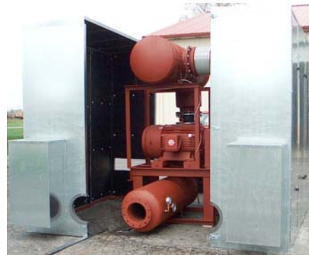
(Above) The lines breaks help identify the many components of the enclosure. (Below) A Typical enclosure would be shipped as a clamshell that clamps around the unit to be enclosed.
